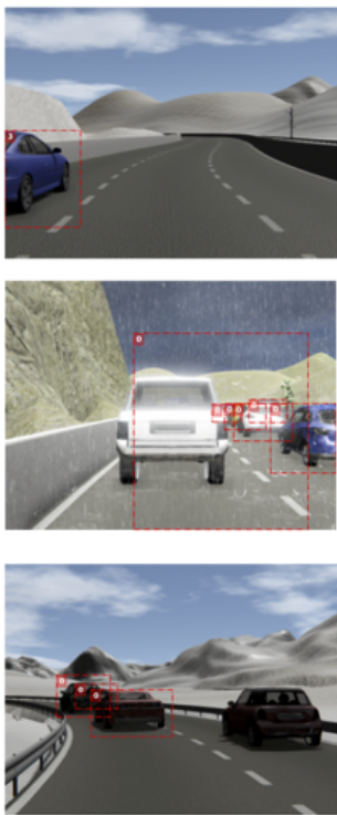
Figure 3. Various errors in our SYNTHIA-AL dataset, including: class label for Car (class #0 in SYNTHIA-AL) swapped with Bicycle (class #3), bounding box around depicted Car shifted to incorrect location (middle), and omitted bounding box around depicted Car (bottom). These examples involve the Car class, but similar errors exist in labels for each of the other 4 classes.
