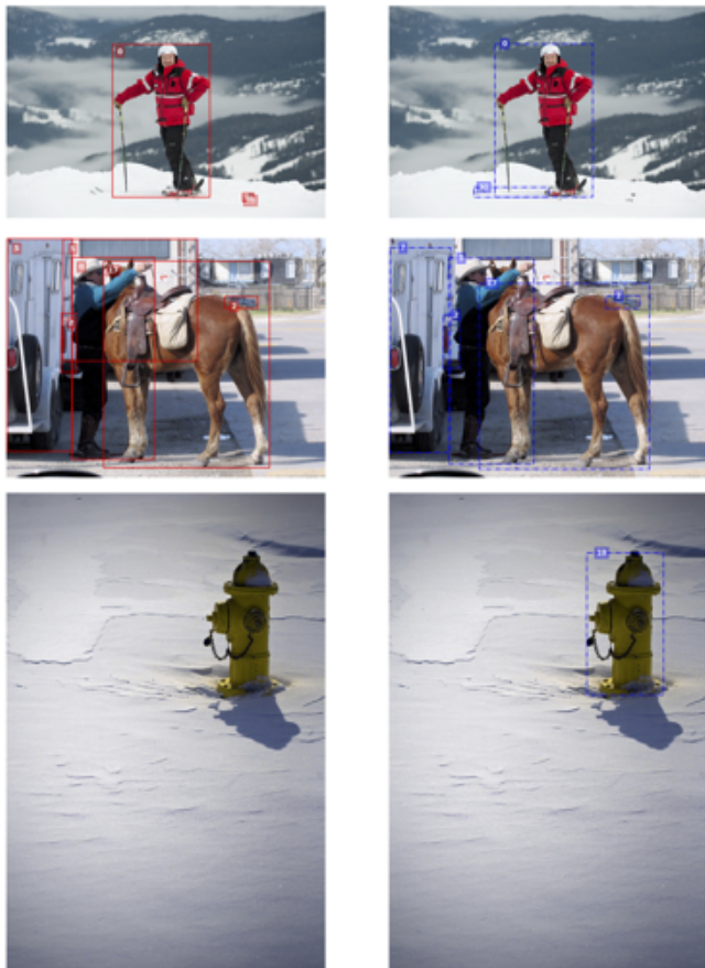
Figure 1. Images in COCO dataset with some of the lowest ObjectLab label quality scores. We show both the original given label (left column in red) and prediction from Detectron2-X101 model (right column in blue). These examples exhibit different naturally-occurring label errors: (top) Overlooked box, (middle) Badly Located box, (bottom) Swapped class label. In top row: annotators poorly outlined the ski (class #30) which the model localized much better (with confidence 0.835), leading to a low Badly-Located score in ObjectLab. In middle row: the vehicle on the left is incorrectly annotated as a bus (class #5), while the model predicted truck with confidence 0.996, leading to a low Swapped-score in ObjectLab. In bottom row: annotators missed the fire hydrant (class #10 in COCO) which the model detected with confidence 0.998, leading to a low Overlooked-score in ObjectLab.
